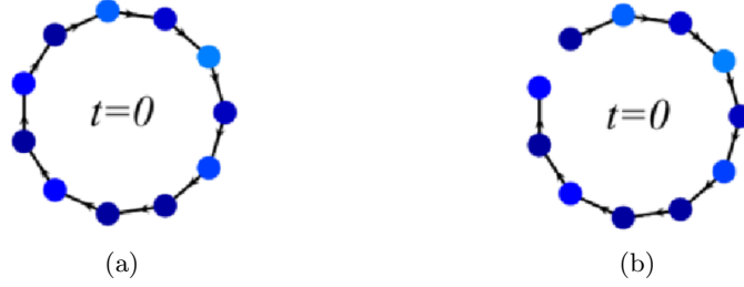
Figure 2: (a) A network with a full rotational symmetry, meaning each vertex has one incoming link and an outgoing one. It is constituted of N = 11 elements. (b) The same network but an edge (at a random place) has been removed.
